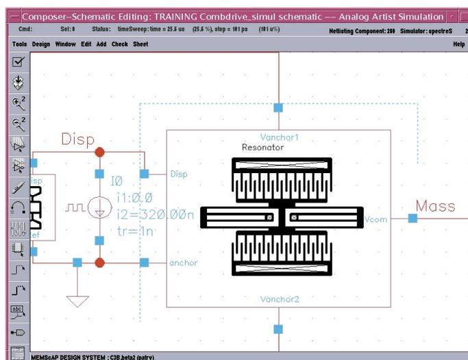
**MEMS Master** is a position dependant schematic tool for rapidly creating hierarchical MEMS models from primitive devices. Models from MEMS Master can then be simulated in the Cadence analog/mixed signal simulator environment ensuring the link with system designers.
