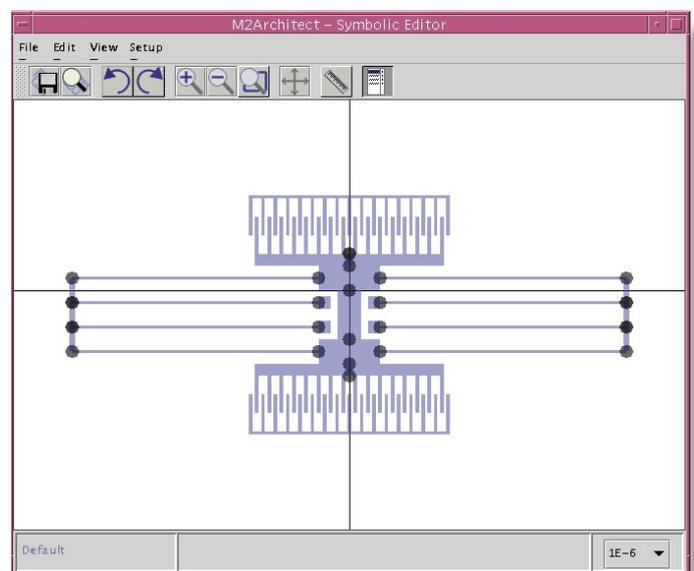
**Modeling:** **MEMS Modeler** automatically generates coupled electro-static-mechanical-thermal behavioral models ready for system simulation with electronics and packaging from 3D data from analysis packages. Complex, finite element models involving a large number of degrees of freedom are reduced to a few master degrees of freedom. Users can also create their own models from analytical equations and the tool generates simulation-ready descriptions in Verilog-A.
